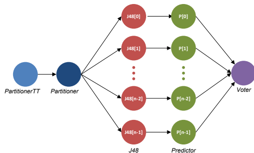
Fig. 11. Task dependency graph associated with the parallel classification workflow.
