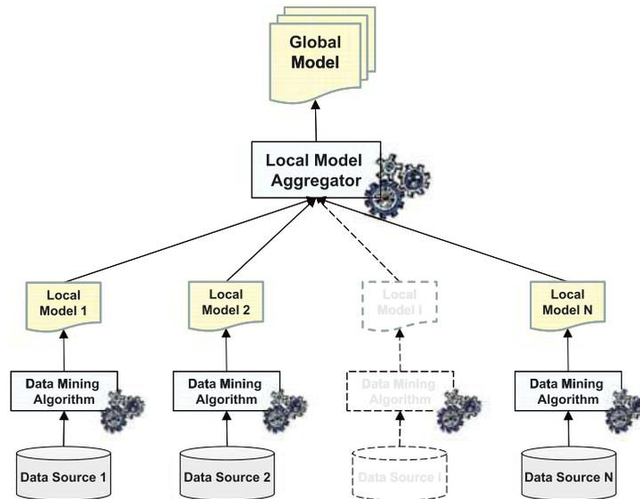
Figure 1. Typical architecture of a distributed data mining algorithm.
