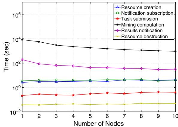
(a) Execution time of the different steps for different number of local nodes, logarithmic scale.
