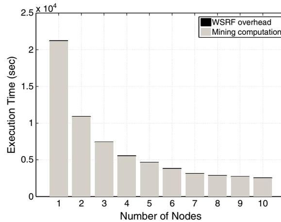
(a) Computation time and WSRF overhead for different number of nodes.
