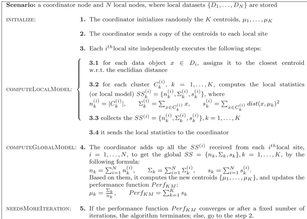
Figure 6. Distributed k-means algorithm.
