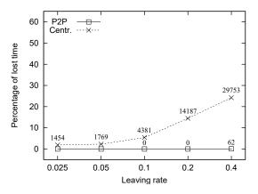
Fig. 6 Percentage of lost time. The numbers in correspondence of each graph point represent the amount of lost computing time expressed in hours.
