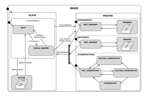
Fig. 3 Behavior of a generic node described by a UML State Diagram.
