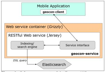
Figure 3 Software components of the Geocon middleware.
