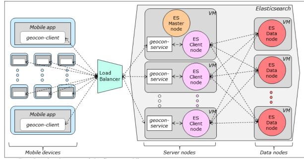
Figure 4 Distributed architecture of the Geocon middleware.
