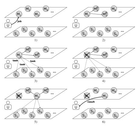
Fig. 3 Steps performed to submit a job and to recover from a master failure
