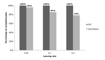
Fig. 6 Percentage of completed jobs in centralized and P2P scenarios for a leaving rate ranging from 0.05 to 0.2
