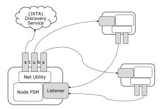
Fig. 5 Software modules inside each node and interactions among nodes in P2P-MapReduce
