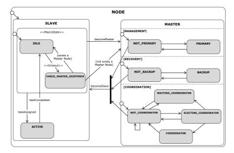
Fig. 4 UML State Diagram describing the behavior of a generic node in the P2P-MapReduce framework
