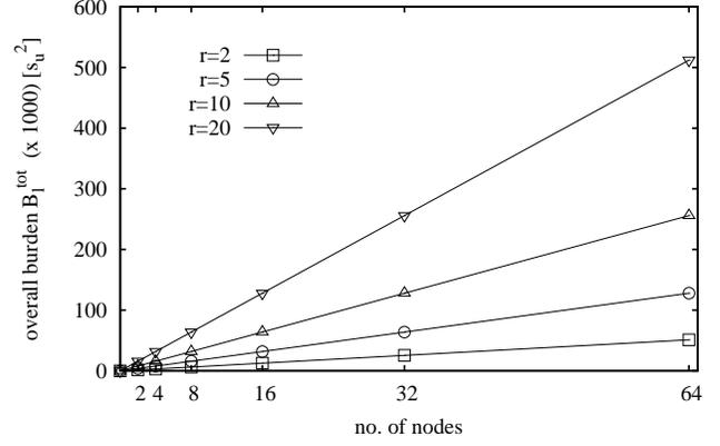
Figure 6. Linear space partitioning: overall burden vs. the number of nodes/regions, for different values of the operational radius.
