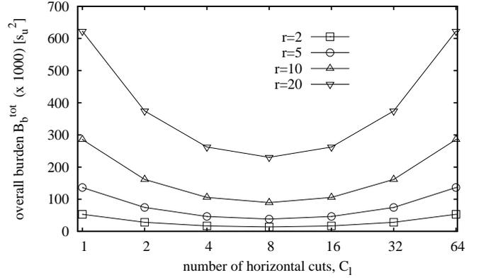
Figure 11. Bidimensional space partitioning: overall burden vs. the number of horizontal cuts  $C_l$ , with 64 regions, for different values of the operational radius.  $N = 64 = C_l \cdot C_h$ . The x axis is in log scale.
