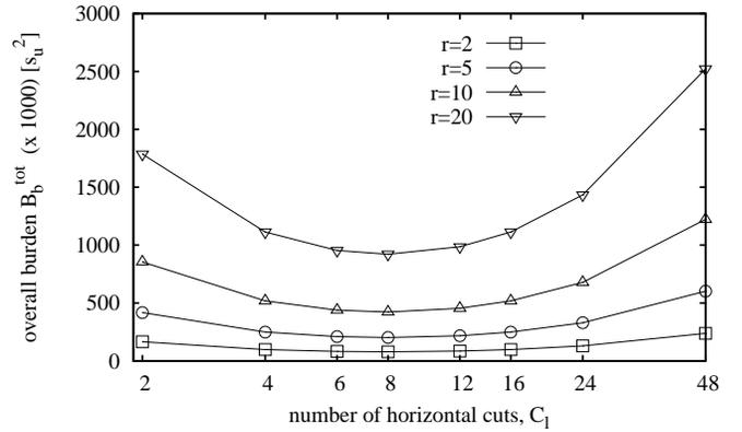
Figure 12. Bidimensional space partitioning: overall burden vs. the number of horizontal cuts  $C_l$ , with 96 regions, for different values of the operational radius, in the case of rectangular territory.  $N = 96 = C_l \cdot C_h$ . The x axis is in log scale.
