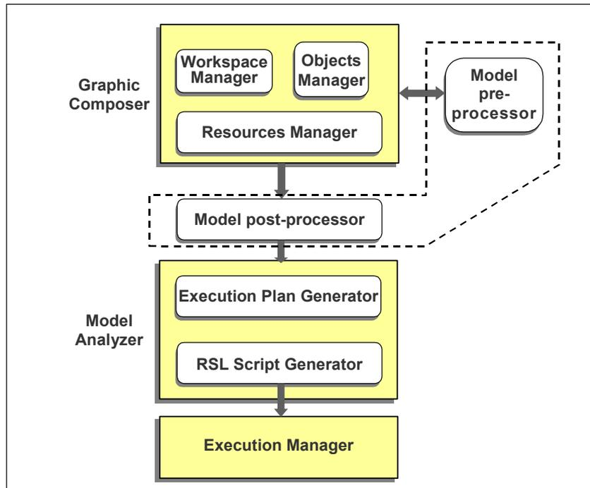
Figure 3: The VEGA software modules.
