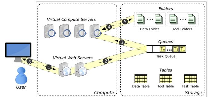
Fig. 1. System architecture and execution steps.
