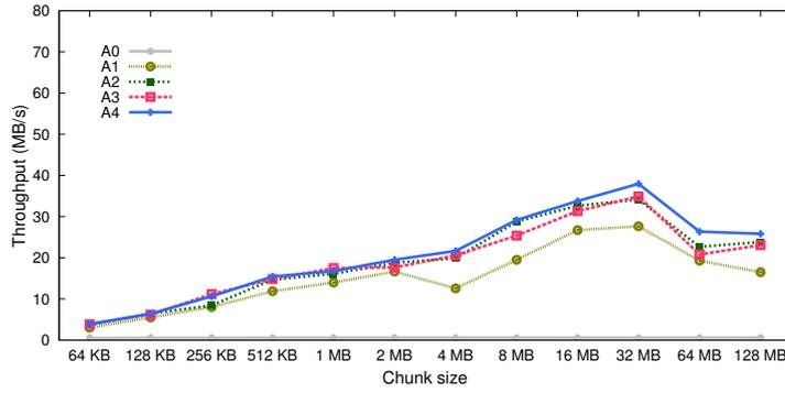
(a) Throughput of Azure Storage by using the Filecopy Benchmark (128 MBytes) for evaluating the block size for writes.
