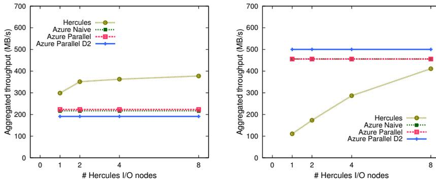
(a) Throughput of Hercules by using the File-copy Benchmark for evaluating the scalability of I/O nodes for writes. We set up the experiment with 8 worker nodes, writing 512 MBytes each one (4 GBytes in total).
