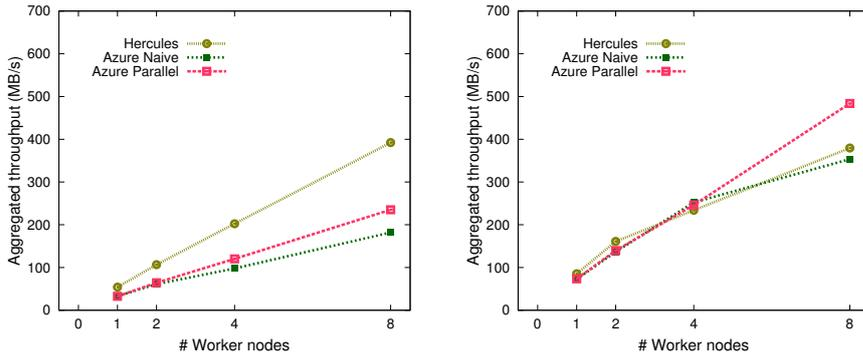
(a) Throughput varying the worker nodes from 1 to 8, writing 8 files (512 MBytes) per node. We set up the experiment with 8 I/O nodes in case of Hercules.
