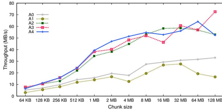
(b) Throughput of Azure Storage by using the Filecopy Benchmark (128 MBytes) for evaluating the block size for reads.
