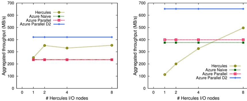
(a) Throughput of Hercules by using the File-copy Benchmark for evaluating the scalability of I/O nodes for writes. We set up the experiment with 8 clients and 4 process per node, writing 128 MBytes each process (4 GBytes in total). (b) Throughput of Hercules by using the File-copy Benchmark for evaluating the scalability of I/O nodes for reads. We set up the experiment with 8 clients and 4 process per node, reading 128 MBytes each process (4 GBytes in total).
