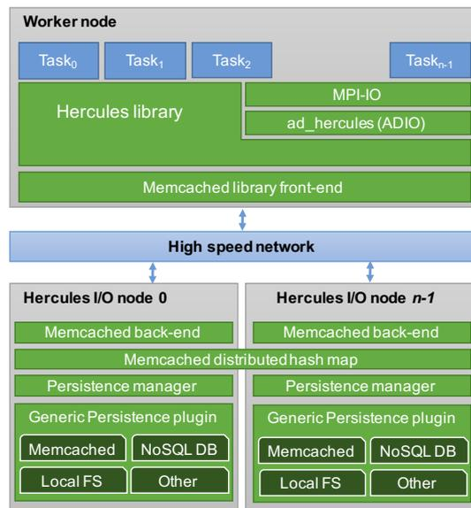
**Fig. 2** Hercules architecture. On the top the worker side, a user-level library. On the bottom the server side with the Hercules I/O nodes divided in modules.
